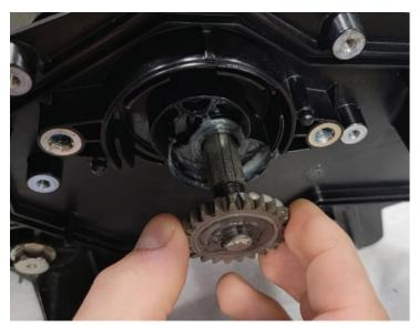
11. Remove the E-clip from the linkage pin. Set the gear shaft linkage aside for later assembly. Figure 13.
