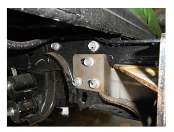
B. With the help of two others mount the bumper to the truck and use the  $\frac{1}{2}$ " stud plates and hardware provided on to the intermediate brackets. Do not fully tighten.
