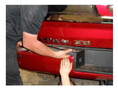
E. Remove tailgate by removing the limit straps and camera harness from the bed. Then pull up on the driver's side of the tailgate with the tailgate approximately halfway open. Then slide the passenger side off the pivot point.
