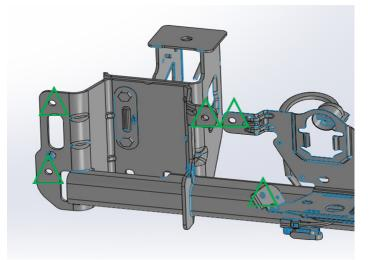
Figure 3c (5x bolt locations per side)
