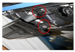
Figure 3b (2x per side, inner bolt locations
