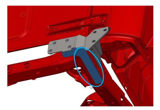
D. After marking the hole locations, remove the passenger side internal and outer frame mounts. With the mounts set aside, drill out the punched locations starting with a 1/4" drill bit, all the way through 5/8".
