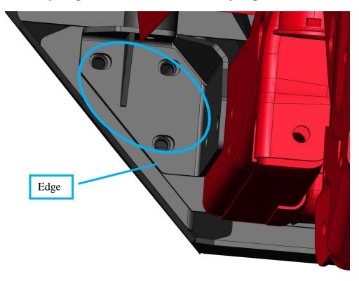
H. With all of the Hardware installed into the Mounts, Frame, and Bumper fully tighten all fasteners using a <sup>3</sup>/<sub>4</sub>" Socket or Wrench.
