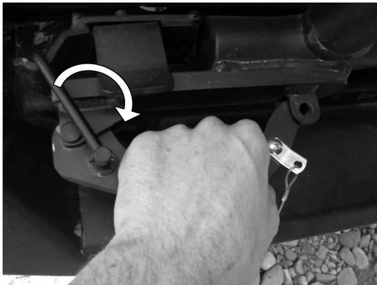
**B. Your tire carrier is equipped with a retaining pin that will hold your tire carrier open when getting items in and out of the back of the vehicle. It, however, is not to be used as a catch for swinging the tire carrier opened uncontrolled for it to engage. Any un-controlled opening could result in damage to the tire carrier itself, the bumper, and possibly the vehicle it is installed on. PLEASE USE CAUTION WHEN OPENING!**
