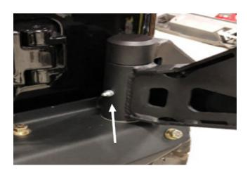
35. Using a 9/16" socket wrench and the provided eight (8) ¾"-16 x 1.25" yellow zinc hex bolt, yellow zinc lock washer, yellow zinc flat washer, fully tighten the two (2) rubber tube stops (61620) to the swing arm (21523). (50173-HW) (Figure 26)
