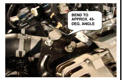
STEP 10: Reinstall alternator bracket and torque bolts to 89 in-lb. Using pliers or an adjustable wrench, bend the tab forward to approximately a 45-degree angle as shown in the figure above. You may need to adjust this angle until there is enough clearance for the alternator wire to clear the intake manifold.
