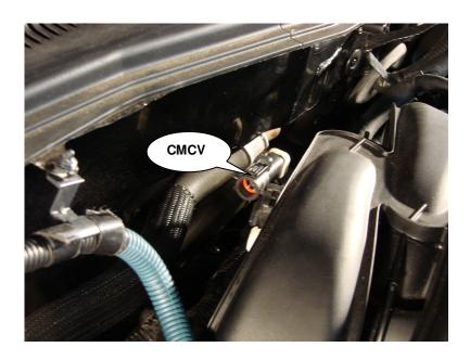
STEP 3: Remove air intake tube or airbox. This requires a 5/16" socket for the clamp at the throttle body.
