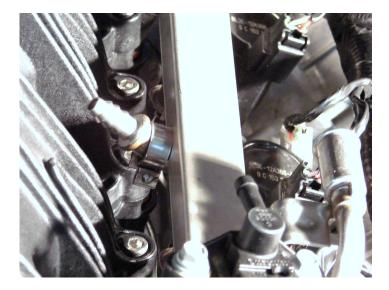
STEP 15: Connect supplied fuel line to nipples on fuel rails using the supplied clamps with a 9/32" socket driver. Do
