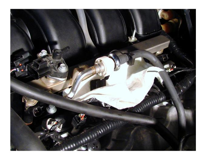
STEP 6: Unbolt fuel rails using an 8mm deep socket. Remove injectors from intake by gently wiggling them while
