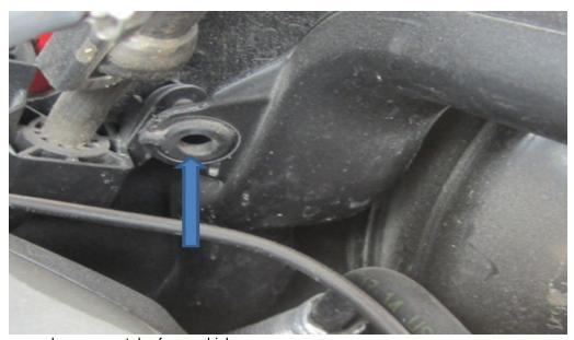
Remove sound symposer tube from vehicle. Install symposer delete plug in engine compartment bulkhead.
