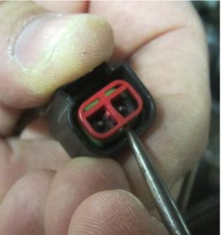
Remove pin lock from new connector.
