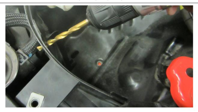
Drill hole for harness retainer.
