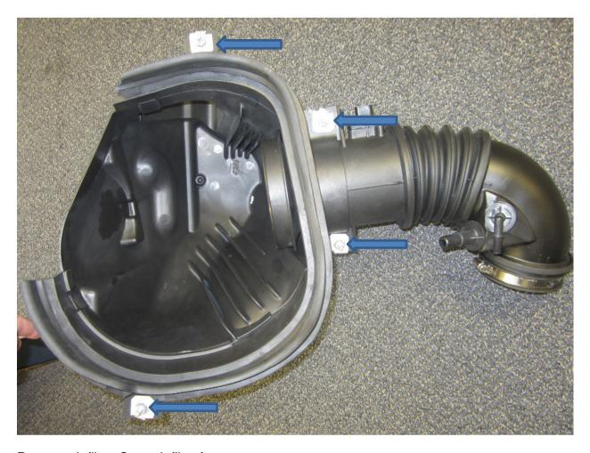
Remove air filter. Save air filter for reuse. Remove air bucket to hood rubber seal from top of air bucket by removing the 4 bolts. Discard air filter to throttle body tube
