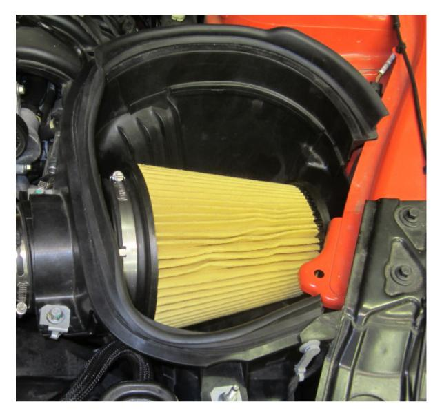
Install air filter. Reinstall air bucket to hood rubber seal using the 4 bolts. Torque to 71 lb. in.
