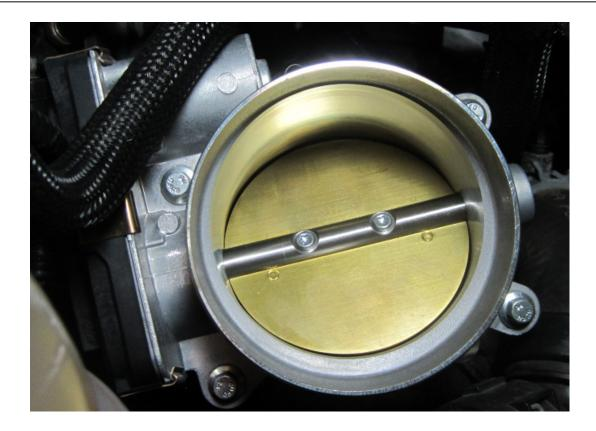
Install the Throttle Body and tighten the Throttle Body retaining bolts. Connect the Throttle Body electrical connector.
