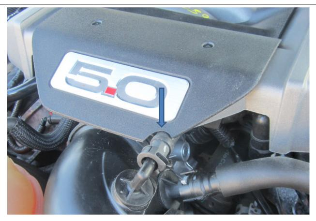
Clearance engine cover as necessary and install.
