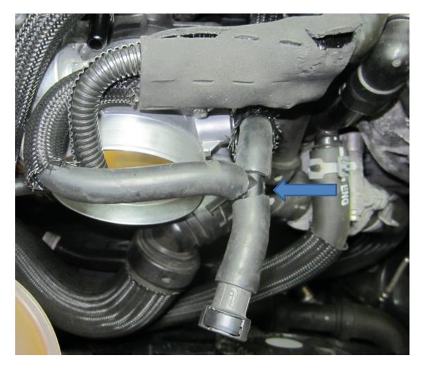
Modify hoses as shown using 3/8 T-connector. (2015-2016 Mustang GT only)
