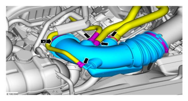
Loosen the clamp and remove the air cleaner outlet pipe. *Torque*: 48 lb.in (5.4 Nm)
