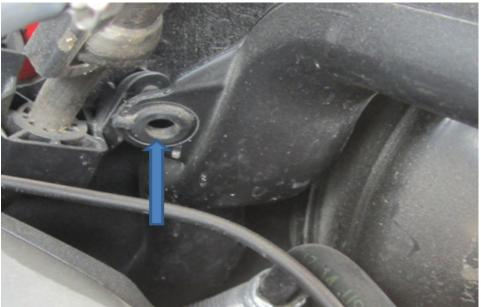
Use a trim panel removal tool or similar to release symposer tube from push pins. Release symposer tube from engine compartment bulkhead.
