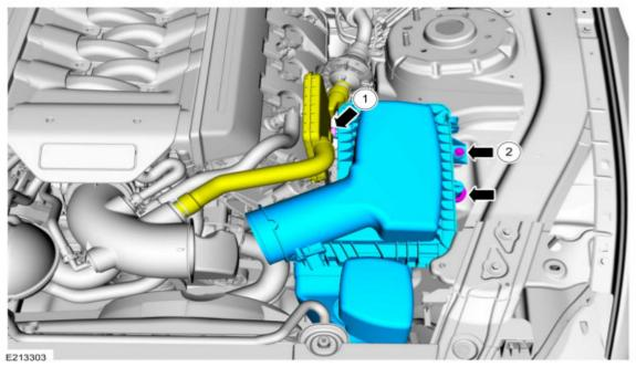
Loosen the clamp and position the air cleaner outlet pipe from the air cleaner.
