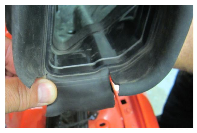
Modify air inlet rubber seal by making two cuts.
