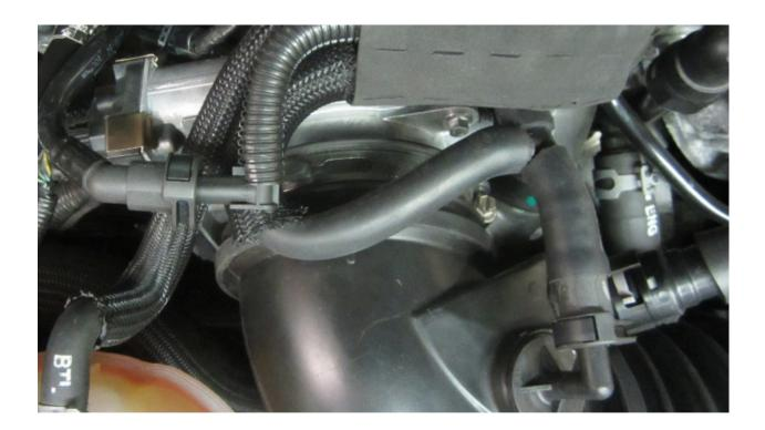
Attach to nipple on air inlet hose.
