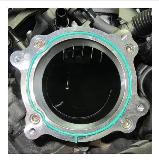
Install throttle body adapter. Torque to 7 ft. lbs.
