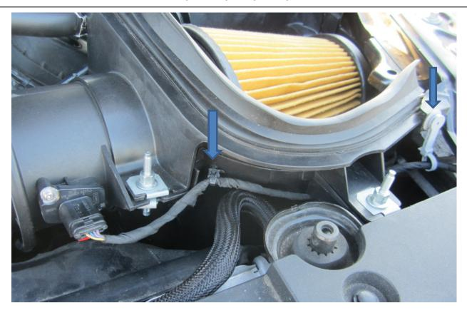
Route MAF harness as shown. Drill hole in Air filter bucket for existing wire tie on harness. Install wire tie with 25mm offset
