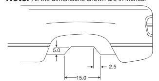
**Note:** The frame depression may be on the upper or bottom half of the frame rail. If your vehicle has an indention on the upper half of the frame use the special flat washers as shown in the illustration directly above.
