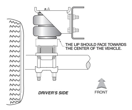
**Notice:** In order to fit this kit on 1987 and prior Chevrolet and GMC two wheel drive 1/2, 3/4, and 1 ton models, the lower bracket needs to be reversed so that the lip on the side of the bracket (as shown in the illustration above) is towards the center of the vehicle.
