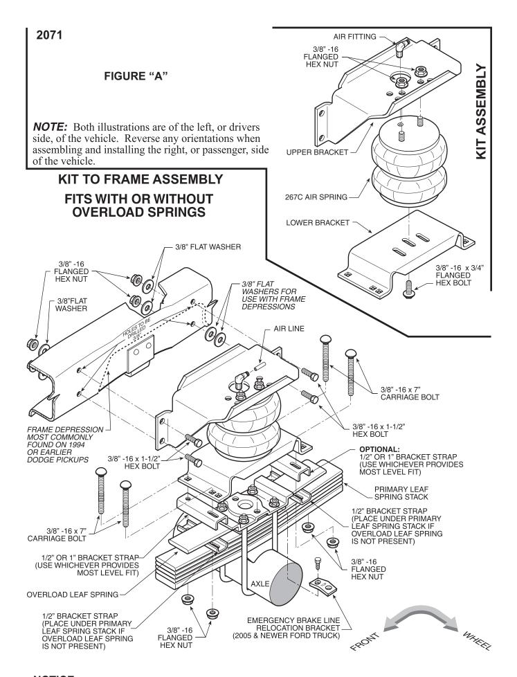
**NOTICE FOR 1973-1987 2WD CHEVROLET AND GMC PICKUPS:** THE LOWER BRACKET NEEDS TO BE REVERSED SO THAT THE LIP ON THE SIDE OF THE BRACKET IS FACING TOWARD THE CENTER OF THE VEHICLE. THE ROTATION OF THE LOWER BRACKET IS TO ENSURE PROPER AIR SPRING ALIGNMENT. THIS APPLICATION ALSO IS USED ON SOME FORD AND DODGE PICKUPS.
