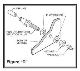
**NOTE:** Too much air pressure in the helper springs will result in stiffer ride, while too little air pressure will allow the air spring to bottom out over rough conditions. Too little air pressure will also not provide the improvement in handling that is possible. **TO PREVENT POSSIBLE DAMAGE MAINTAIN A MINIMUM OF 5 P.S.I. IN THE RIDE-RITE AIR SPRINGS AT ALL TIMES.**
