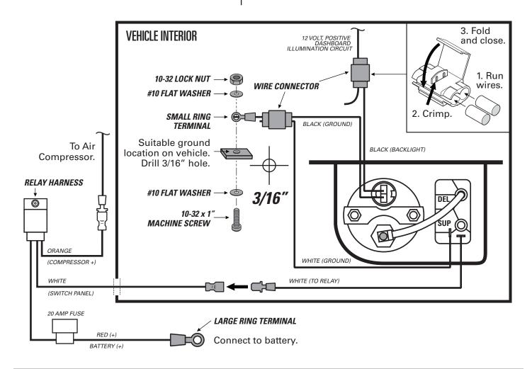
Install the Control Panel using the supplied fasteners.
