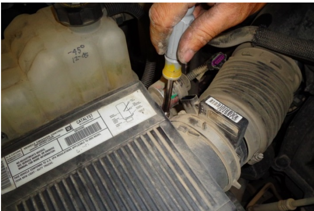
8. Loosen the screw clamp securing the MAF sensor to the airbox.
