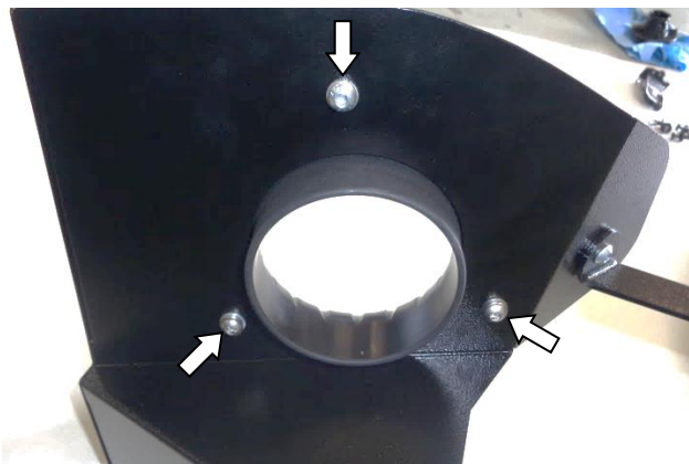
21. Assemble air filter adapter (3) to heat shield using M6 screws (6), lock washers (5) and flat washers (4).
