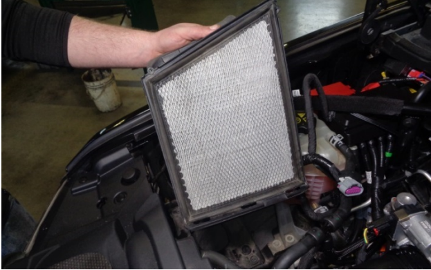
13. Remove the airbox from the vehicle by pulling it firmly straight up to release it from its rubber grommets.
