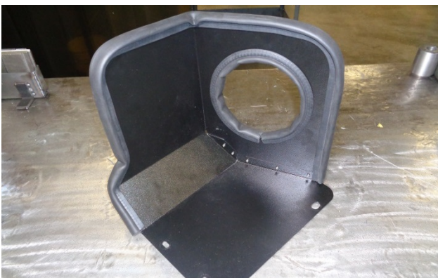
15. Attach the gasket (4) to both the opening and the outer edge of the heat shield (3) as shown. Firmly press the gasket onto the edge, gradually working all the way around. At the end point, use metal-cutting shears to trim the gasket to fit.
