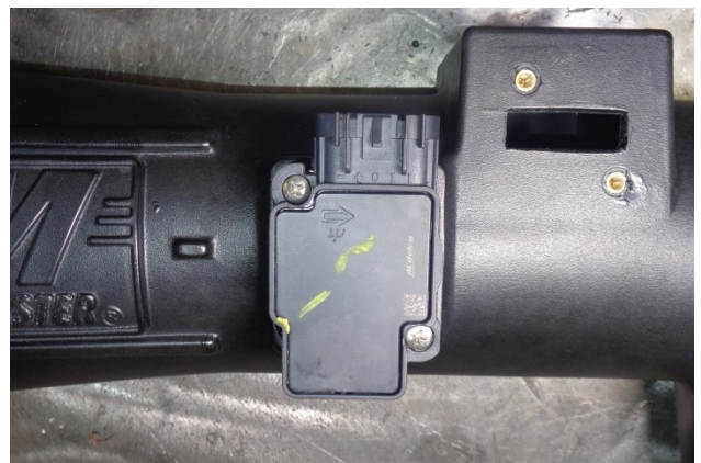
18. Install the MAF sensor gasket (7) on the sensor, ensuring correct orientation. Then install the sensor in the intake tube, using the long M4 screws (9).
