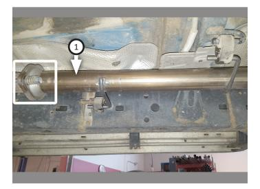
8. Place **clamp (5)** onto **muffler (2)** then connect it to inlet pipe. Tighten clamp just enough to allow for adjustment then place another **clamp (5)** onto muffler outlet.
