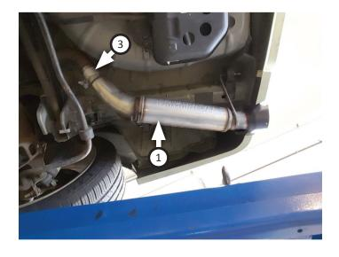
6. Place clamp (3) onto left muffler assembly (2) and seat it 2" deep into left tailpipe. Insert (x2 ea.) wire hangers into isolators then tighten clamp just enough to allow for later adjustment.
