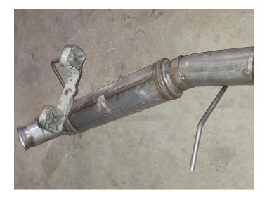
5. Place clamp (removed step 3) onto **right muffler assembly (1)** then connect it to right exhaust outlet. Insert wire hangers into isolators and tighten clamp just enough to allow for later adjustment.
