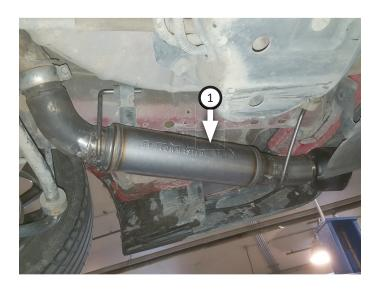
Place clamp (removed step 3) onto left muffler assembly (2) then connect it to left exhaust outlet.
