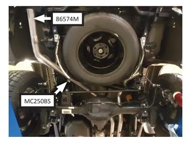
15. Place **clamp (M250BS)** onto **right exit pipe (86575M)** then connect it to right overaxle pipe. Insert wire hanger into isolator then tighten clamp just enough to allow for adjustment.
