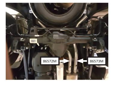
14. Place **clamp (M250BS)** onto **left exit pipe (86574M)** then connect it to left overaxle pipe. Insert wire hanger into isolator then tighten clamp just enough to allow for adjustment.
