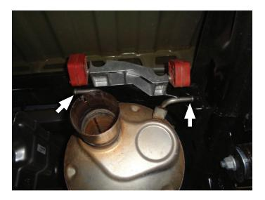
6. Disassemble nuts (x2) from factory pipe and catalytic converter flange. Remove muffler and factory pipe from vehicle.
