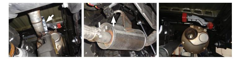
5. Remove factory muffler wire hangers (x3) from factory isolators and detach grounding wire.
