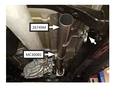
12. Place clamp (MC300BS) onto muffler (72288-Z) inlet, then connect muffler to extension. Tighten clamp on muffler inlet just enough to allow for adjustment. Place clamps (x2) (MC250BS) onto muffler outlets.
