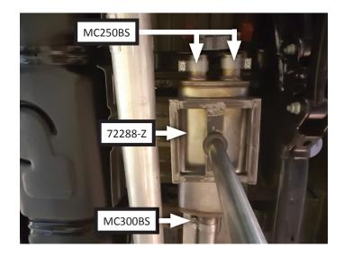
13. Route **right and left overaxle pipes (86537M, 86572M)** over axle and connect them to muffler outlets. Mount wire hangers into isolators then tighten clamps (x2) enough to allow for adjustment.
