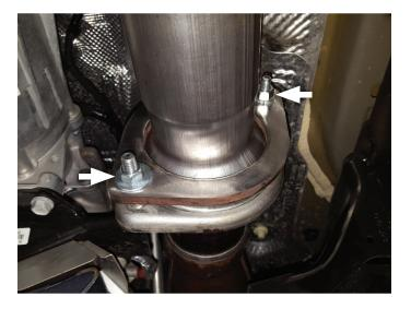
11. Place clamp (MC300BS) onto extension pipe (26749M) then connect them to inlet pipe. Insert wire hanger into isolater and plug in grounding wire (removed step 5). Tighten clamp just enough to allow for adjustment.
