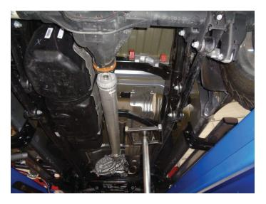
7. Remove stock studs from catalytic converter flange.
