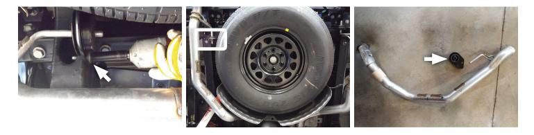
5. Cut tailpipes just behind factory muffler.
