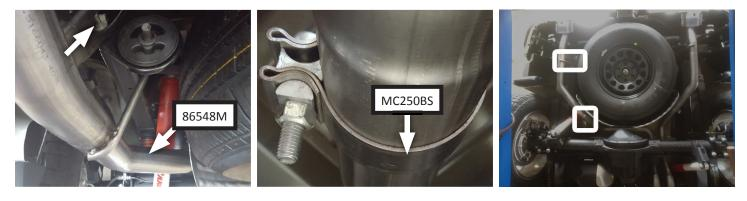
16. Adjust exhaust components to provide a satisfactory fit. Maintain a minimum of ½" clearance around all components of exhaust system, keeping in mind suspension, travel and vibration. After making any required adjustments, securely tighten clamps.
