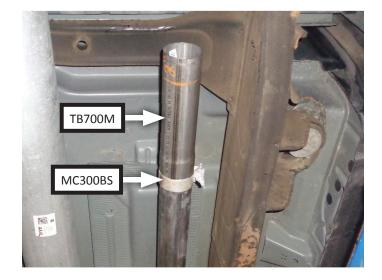
12. Place clamp (MC300BS) onto muffler (72288-Z) inlet. Place clamps (x2) (MC250BS) onto muffler outlets. Connect muffler to inlet or extension pipe then tighten front clamp just enough to allow for adjustment.
