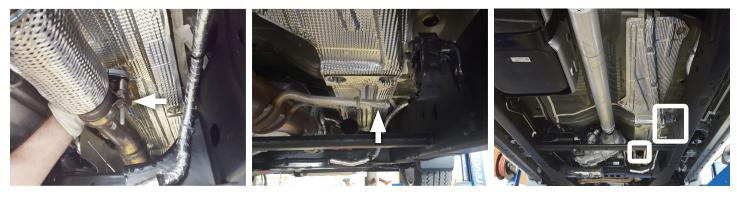
8. Release tab and remove factory clamp from pipe inlet. Retain factory clamp for later use.
