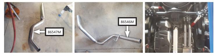
14. Place clamp (MC250BS) and mount (removed step 6) onto right rear tailpipe (86549M) then connect it to right front tailpipe. Bolt mount onto frame then tighten clamp enough to allow for adjustment.
