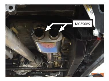
Route right front tailpipe (86547M) and left front tailpipe (86546M) over axle and connect them to muffler outlets. Mount wire hangers into isolators then tighten clamps (x2) enough to allow for adjustment.
