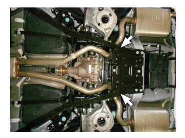
4. Measure and mark 2½" from beginning of straight section on exhaust pipes (x2) as shown. Support then cut pipes at marks. Unbolt hanger mounts and remove tailpipes from vehicle.
