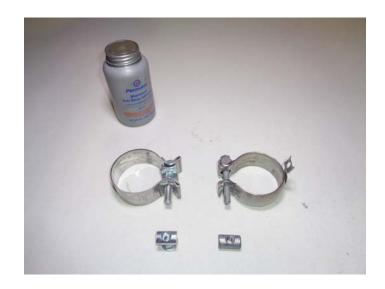
www.flowmastermufflers.com Technical Support (866) 464-6553 7. Place **clamp (6)** onto **inlet pipe (1)** then connect it to catalytic converter. Insert wire hanger into isolator and tighten clamp enough to allow for adjustment.
