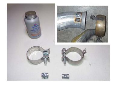
7. Place factory ball clamp (removed step 5) onto **muffler assembly (1)** then connect it to cat. converter. Tighten clamp enough to allow for adjustment.
