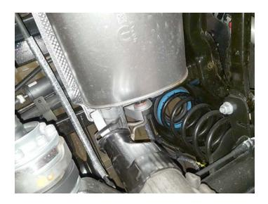
4. Support muffler and disassemble wire hangers from isolators. Loosen ball clamp, disconnect inlet pipe at cat. converter and remove exhaust system.
