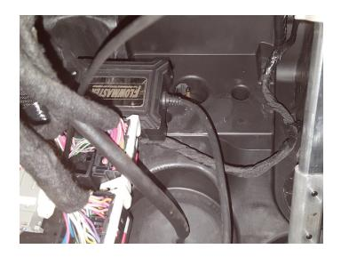
17. Strip end of controller kit red wire. Connect **fused circuit** tap (17) to it then crimp connection.
