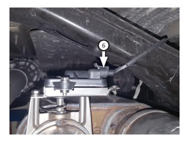
**NOTE:** You may secure wire assembly several different ways; **zip tie (15)** it to factory wire bundle, tuck it behind heat shield, secure it to frame, etc. Just be sure that connections are stable and wire is protected from heat.
