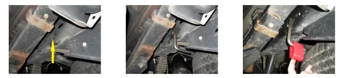
11) Place a provided 4" clamp onto the expanded end of pipe **#46174S**, connect the hanger on the pipe to the rubber mount installed in the step above. Then connect the front of the pipe to the rear of pipe **#46172S**. Confirm that the two pipes are fully slid together and tighten the clamp enough to hold, but still allow for adjustment.
