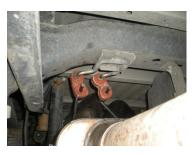
6) Place a supplied 4" clamp onto the inlet of muffler **#8540152-Z** and slide onto the back of inlet pipe **#TB425S** or extension pipe **#46184S**. Tighten the clamp enough to hold, but still allow for adjustment.
