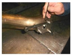
2) The mount with the spacers and washers attached. Tighten securely.
