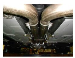
5) Begin the installation by placing a supplied 2-3/4" clamp onto each of the inlets of the Scavenger pipe #26591S. Then place the Scavenger pipe onto the back of the stock head pipes (the offset outlet pipe should be oriented to the passenger side). Level and center the assembly in the drive line tunnel and support with a stand. Tighten the two clamps enough to hold, but still allow for adjustment.
