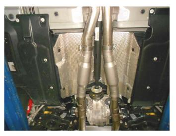
Place a supplied clamp onto the left muffler outlet. Place the left tailpipe # 26654S into position and starting from the rear, connect the hangers on the tailpipe to the rubber mounts on the vehicle. Slide the tailpipe fully into the muffler outlet and adjust the tailpipe so that the end of the pipe is centered in the factory exhaust bezel. See photo below. Tighten clamp enough to hold, but still allow for adjustment. Repeat this step for right tailpipe # 26652S.
