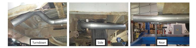
www.flowmastermufflers.com Technical Support (866) 464-6553  Place clamp (14) onto left (9) and right (10) exit turndown pipes then connect them to muffler exit. Tighten clamps just enough to allow for adjustment.
