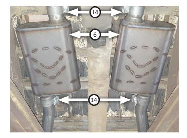
**NOTE:** For short and long bed vehicle models, trim tailpipes depending on exit pipe placement and preference.
