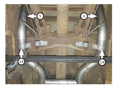
**NOTE:** If factory holes are not present, skip this step, the hanger will be installed later.
