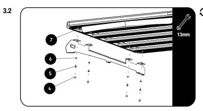
Fit your Roof Rack to the Foot Rails using M8x20 Hex Bolts, M8x16x1.6SS Flat Washers and M8 Nyloc Nuts (Items 7, 6 & 5) as shown.
