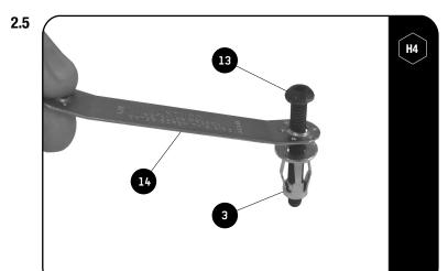
Insert the M6 Button Head Bolt (Item 13) into the one side of the Jack Nut Tool (Item 14). Loosely fit a Jack Nut (Item 3) to the Button Head Bolt as shown. Using the Jack Nut Tool and a M6 x 30 Button Head Bolt, insert the M6 Jack Nuts into all 8 holes. Place the assembly into the hole drilled. Using a Battery Powered Screw Driver and a H4 Allen Key Bit, set the Jack Nut into the hole while holding onto the handle of the Jack Nut Tool.
