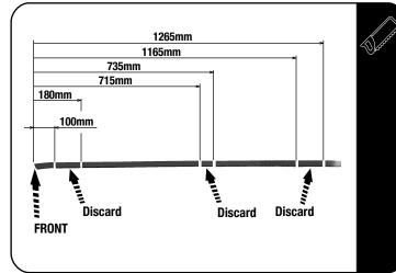
Lay the left-hand ditch moulding on an even surface. From the front tip of the ditch moulding, measure and mark as shown.
