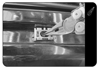
Remove all the retaining clips using a long nose plier as shown.
