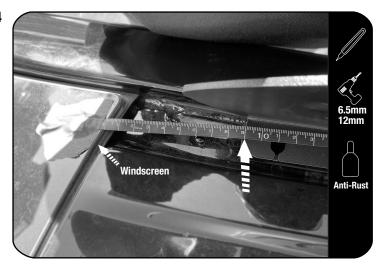
Place the Spacers (Item 2 & 12) in the ditch and place the Foot Rail (Item 1) on top with the Spacers (Item 2) under the front and rear Foot mounts and Spacer (Item 12) under the single Foot mount. Position the Foot Rail 90mm from the top edge of the windscreen as shown. Centralize the slotted holes in the Spacers with the slotted holes in the Foot Rail feet.
