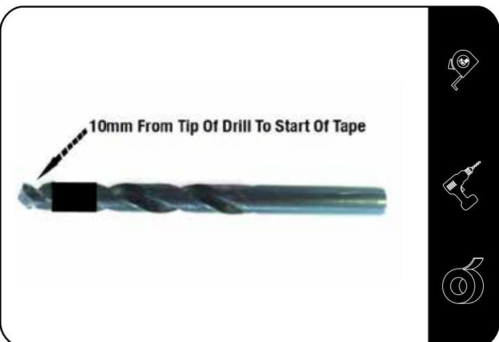
Before drilling the holes in the roof, take both 4 & 9 mm drill bits and wrap a band of insulation tape around the drill bits to act as a stopper to prevent you from drilling to deep as there are airbags located below where you will be drilling.
