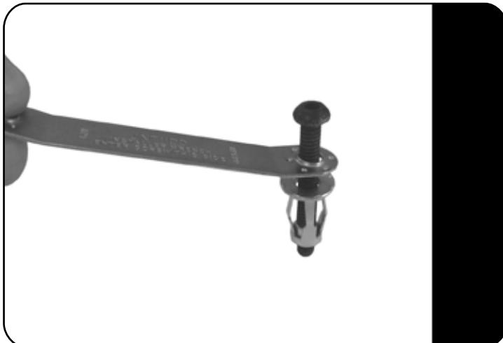
Insert a M6 button head bolt (Item 15) into the side of the installer wrench (Item 14). Loosely fit a jack nut (Item 7) to the button head bolt as shown.
