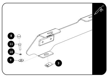
Before fitting the Foot Rails to the vehicle, ensure the factory hole threads are clean and free from any dirt or debris.
