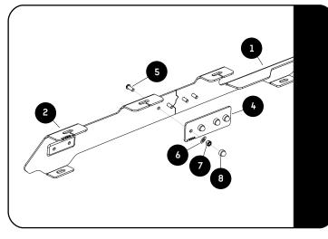
Loosely join the Front and Rear Foot Rails (Items 1 & 2) together using M6 x 16 Button Head Bolts, M6 x 12 x 1 Flat Washers, M6 Nyloc Nuts and the Joiner Plate (Items 5, 6, 7, 8 & 4) as shown.
