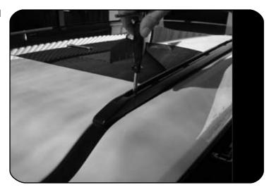
Using your torx wrench, loosen and remove the original factory tracks. If your vehicle did not come with these tracks, refer to 2.4.
