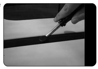
Use a small flat screwdriver and remove the plastic cap in the front ditch molding on either side of the sun roof to expose the threaded mounting points.
