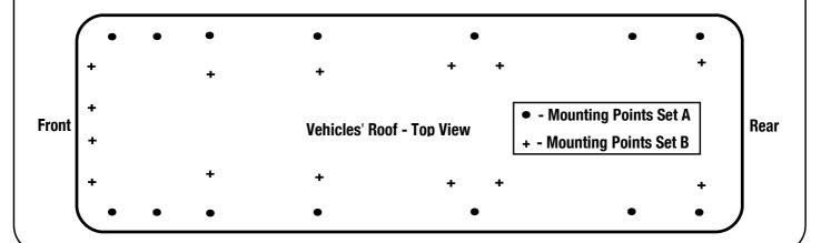
( C ) Place the left and right hand side Front Foot Rails (Item 5) onto the vehicles' roof, lining up the mounting points in the Foot Rails with the first three mounting points in the front of the vehicles' roof.
