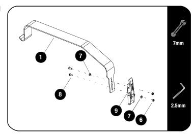
If needed, adjust the Latch (Item 9) using two M4 x 10 Button Heads, two M4 Flat Washers and two M4 Nyloc Nuts (Items 6, 7 & 8) before fully tightening.
