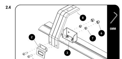
Assemble the Legs (Item 8) to the Leg Mount (Item 3) by using M8 x 25 Button Heads and M8 nyloc Nuts (Items 4 & 7) and the M8 x 20 T-Bolts (Items 1).
