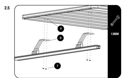
Loosely fit your Slimline II Rack by using M8 x 25 Hex Bolts and M8 Nylocs (Items 7, 9) as shown.
