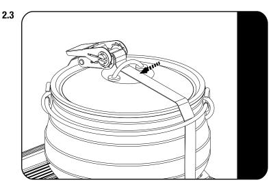
Secure the Potjie Pot / Dutch Oven using the Ratchet Strap, the strap should go through the lid as shown.
