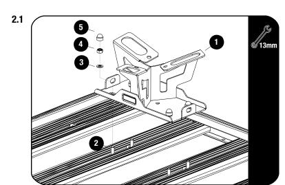
Decide where on the rack you would like to mount your Potjie Pot / Dutch Oven Holder, the Potjie Pot / Dutch Oven Holder needs to be mounted across two slats as shown.
