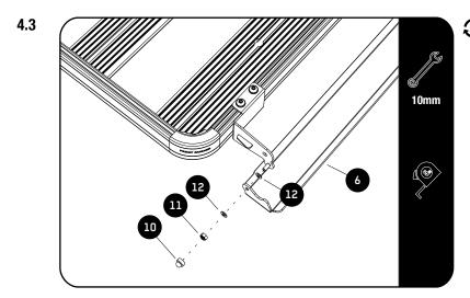
Fasten the Front Cover (Item 6) to the two Mounting Brackets using M6 x 12 x 1SS Flat Washers and M6 Nyloc Nuts (Items 12 & 11). The Front Cover should still be able to rotate after fastening.
