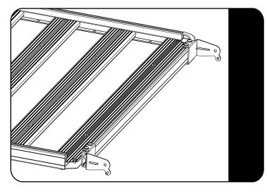
Slide the both Front Mount Brackets into the Combined Slat as shown.
