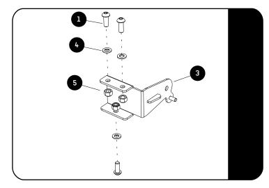
Assemble the left and right Front Mounting Brackets (Item 3) the M8 x 20 Button Head Bolts, M8 x 16 x 1.6SS Flat Washers and M8 Nyloc Nuts (Items 1, 4 & 5) as shown.
