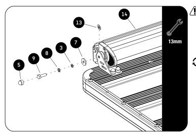
Test fit the Light Bar between the two brackets. If there is a gap between the light and the brackets use Item 13 to fill the gap. This will prevent the Light Cover from bowing.
