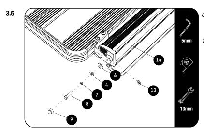
Test fit the Light Bar between the two brackets. If there is a gap between the light and the brackets use Item 13 to fill the gap. This will prevent the Light Cover from bowing.
