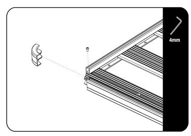
Remove the front right hand side corner piece of the Rack.
