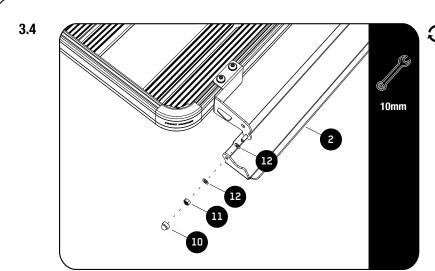
Fasten the Front Cover (Item 2) to the two Mounting Brackets using the four M6 Flat Washers and two M6 Nyloc Nuts (Items 12 & 11). The Front Cover should still be able to rotate after fastening, but should not open on its own.
