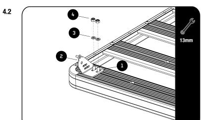
Loosely fasten the two Mounting Brackets (Item 2) to the front slat of the rack, using the M8 x 20 Hex Bolts (Inserted in 4.1), M8 x 16 x 1.6SS Flat Washers and M8 Nyloc Nuts (Items 3 & 4).
