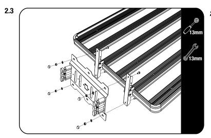
Fit the Rotopax mounting plate to the Rotopax side mounting brackets. Move the side mounting brackets to the desired position before fully tightening all the fasteners.
