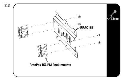
Fit 2 RotoPax RX-PM mounts to the RotoPax mounting plate (RRAC157). Fasteners are supplied with the RotoPax RX-PM pack mounts
