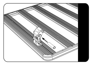
For fork & wheel sets fitted with Boost Hubs. Insert Boost Hub insert into 20mm tube.
