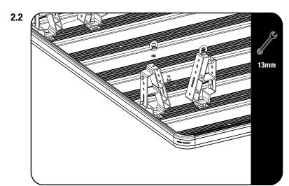
To transport BULKY cargo, use two pairs of Mounting Bracket.
