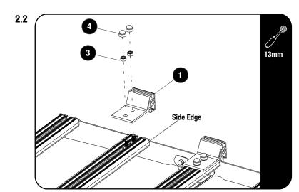
Loosely assemble the Mounting Brackets (Item 1) onto the slats using four M8 Nyloc Nuts (Items 3) as shown.
