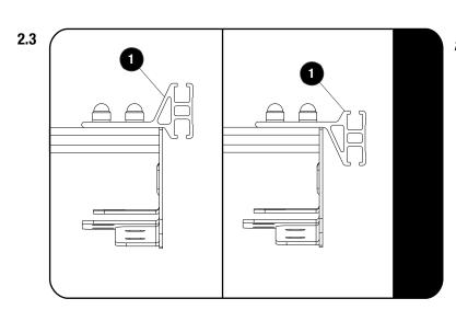
The Mounting Brackets (Item 1) orientation is roof rack accessory dependant.
