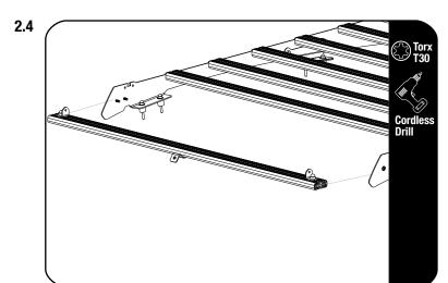
Secure the assembly from step 2.3 to the front two bottom holes on the Foot Rails using the fasteners removed in Step 2.1. Fully tighten.
