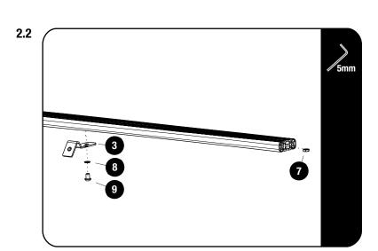
Remove the Wind Fairing Mid Support Bracket that is currently on the slat and replace it with the Fairing Mid Support Bracket supplied with this kit (Item 3).
