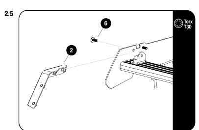
Secure the Wind Fairing Side Supports LH / RH (Item 2) to the Foot Rail's top holes as shown using M6 x 16 Flange Button Head (Item 6).
