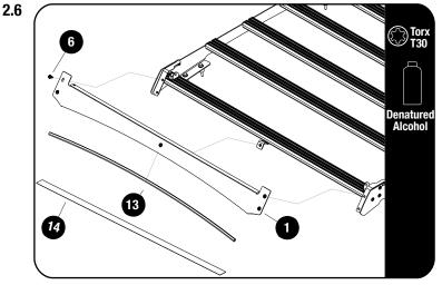
Fit the Wind Fairing Rubber (Item 13) to the Wind Fairing (Item 1). Using the notched section as a guide, trim if needed.
