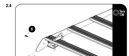
Secure the Wind Fairing Side Supports LH / RH (Item 2) to the foot rails top holes as shown using M6x16 Flange Button Head (Item 6).
