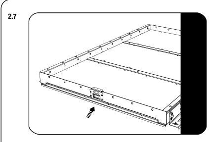
Refer to Step 2.2, refit the tray and stoppers. Once refitted check that the push to close latch engages fully and that the slide is secure.
