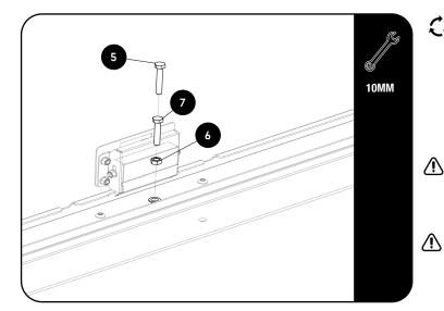
Before refitting the slide to the frame, use the M6 x 35 or M6 x 40 hex bolt (Item 5 or 7) (depending on which fits the specific vehicle best) together with the M6 Normal nut(Item 6) and assemble as shown.
