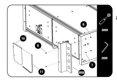
Secure the Front Faces (Item 4 or 10) to the drawer using M5 x 12 Button Heads, M5 Flat Washers and M5 Nyloc Nuts (Items 6, 7 & 8) as shown.
