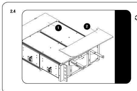
Fit the LH and RH Side Decks (Items 1,2 or 3) to the drawer by placing them into the C-Clips and pushing down on the drawer side.
