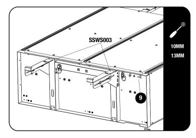
Assemble and fit the Wing Set (SSWS003) to the drawer. Refer to SSWS003's fitting Instruction for assembly.
