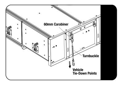
To secure the front of the drawer use 60mm Carabiners and Turnbuckles supplied with SSDR005.
