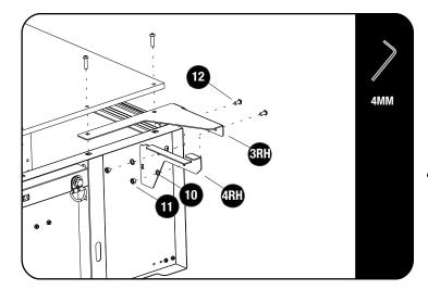
Loosen the rear deck of the drawer. Place the Rear Wing (Item 3) between the deck and the drawer.
