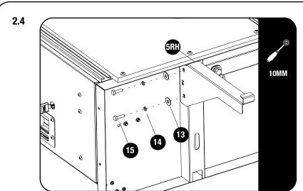
Secure the Front Wings (Item 5) using M6 x 20 Hex Bolt, M6 Spring Washers and M6 x 19 x 1SS Flat Washers (Items 13, 14 & 15) as shown.
