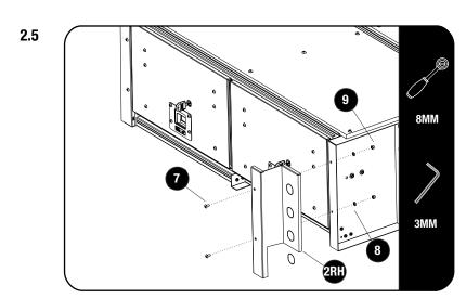
Secure the Front Faces (Item 2) to the drawer using M5 x 10 Button Heads, M5 Flat Washers and M5 Nyloc Nuts (Items 7, 8 & 9) as shown.
