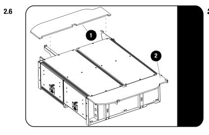
Fit the LH and RH Side Decks (Items 1 & 2) to the drawer by placing them into the C-Clips and pushing down on the drawer side.
