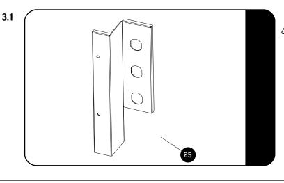
Twist the pre cut knock outs to remove. These cut outs can then be used to fit Front Runners range of electrical sockets.
