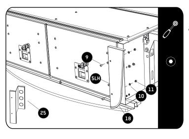
Secure the Front Faces (Item 18 or 25) to the drawer using M5 x 12 Button Heads, M5 Flat Washers and M5 Nyloc Nuts (Items 9, 10 & 11) as shown.
