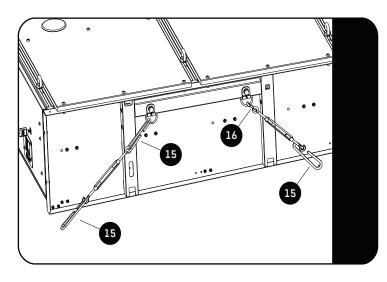
Place the Drawer in the vehicle. Using the Side Decks, position the drawer in the vehicle. See Step 2.6.
