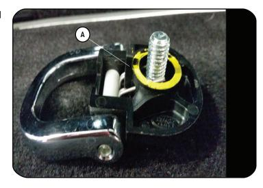
Looking just inside the rear door, loosen the left and right tie-down ring. Cut the plastic locating strip (A) off with a Side Cutter.
