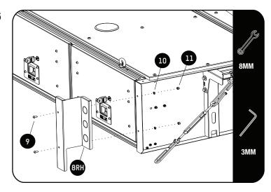
Secure the Front Face (Item 8) using M5 x 10 Button Heads , M5 x 10 x 1SS Flat Washers and M5 Nyloc Nuts (Items 9, 10 & 11)
