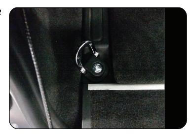
Refit the tie-down rings facing outward as shown.
